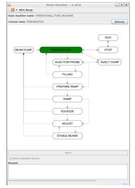
Figure 1: LHC Operational States diagram in SM GUI.
