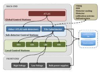
Figure 1: Hierarchy of the DCS of the Tile Calorimeter, as part of the ATLAS control system.
