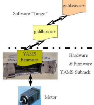
Figure 5: Hardware/Software Architecture.
