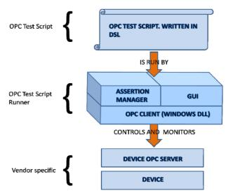
Figure 1: OPC Test Script Runner Components.
