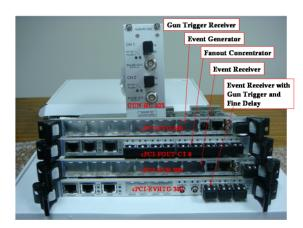
Figure 2: TPS timing modules.
