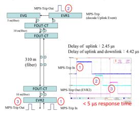
Figure 6: Timing measurement of uplink and downlink with 310 m fiber and three stages of fan-out concentrator.
