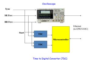
Figure 5: Timing system healthy monitoring. Based upon the reports of several light sources, there are several tens of psec drift around the year. This is acceptable for most of the accelerators timing and users timing requirement. However, to measure the timing drift of specific links, several approaches can be used.
