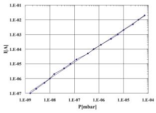
Figure 2: 25lps noble diode ion pump, Uconst=7kV.
