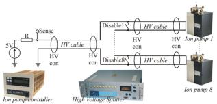
Figure 6: Cable Interlock diagram for one ion pump controller, HVS and 8 ion pumps.
