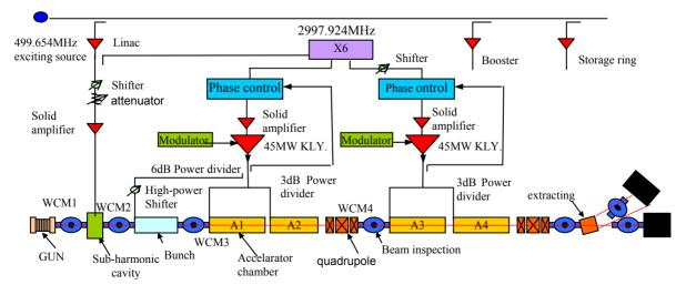
Figure 2: 150MeV Linac RF system layout.
