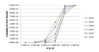
Figure 4: Probability of *False trigger* against  $\lambda f$  between 1E-7 h<sup>-1</sup> and 1E-2 h<sup>-1</sup>
