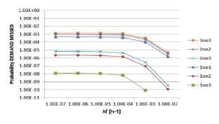
Figure 6: Probability of *Demand missed* against  $\lambda f$  between 1E-7 h<sup>-1</sup> and 1E-2 h<sup>-1</sup> (logarithmic scale).
