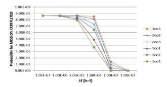
Figure 5: Probability of Mission completed against  $\lambda f$ between 1E-7  $h^{-1}$  and 1E-2  $h^{-1}$ .
