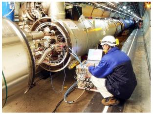
Figure 2: High Voltage qualification in the LHC tunnel.
