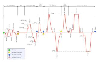
Figure 1: Current cycles for 600A circuit validation.
