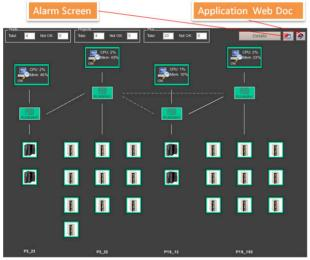
Figure 4: MOON user interface showing the layout of the cryogenics control applications for Point 2 of the LHC.
