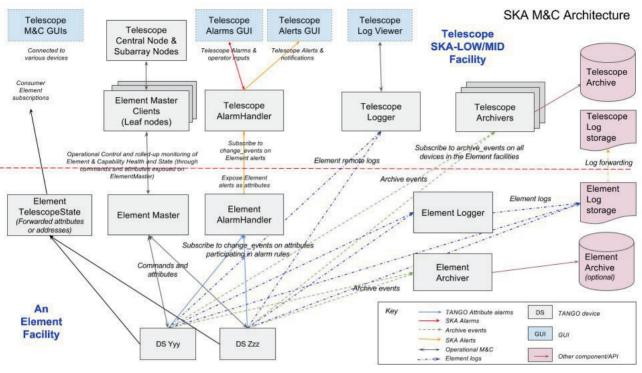
Figure 1: Proposed monitoring and control architecture.
