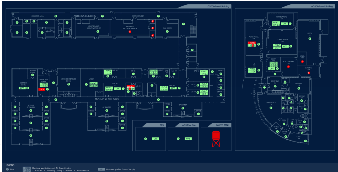
Figure 7: Mock-up interface for the alarms generated by the building infrastructure of the ALMA observatory.
