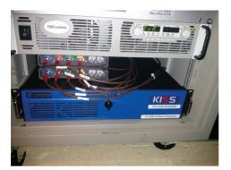
Figure 6: FEC and oscilloscopes used for arc detection in LHC.
