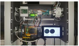
Figure 6: one of the ALICE  $O^2$  simulator setups, with Raspberry Pi, Arduino and sensors installed on the top rail, and DC-DC converters and a User Interface touchscreen on the bottom rail.
