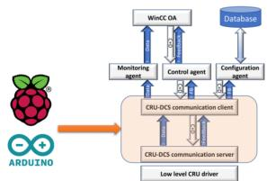
Figure 5: In absence of the CRU (Common-Readout-Unit) and Front-End cards, a Raspberry Pi and Arduino based setup is the proof of concepts for the DCS role into the new read-out chain.
