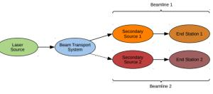
Figure 1: Simplified view of a laser system.
