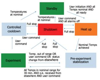
Figure 4: Vapour source simplified control system states.
