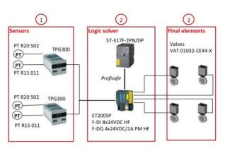
Figure 7: Safety instrumented function architecture.
