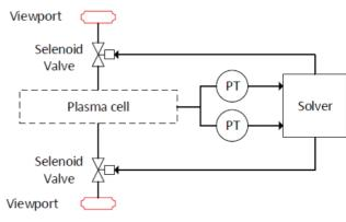
Figure 6: Safety instrumented function Loop.
