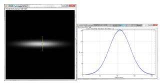
Figure 5: EPICS V4 ImageJ Display and Live Gaussian Profile Fit and Plot.
