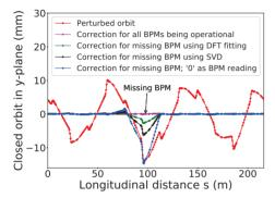
Figure 7: Comparison of SVD and DFT based orbit correction in case of missing BPM.
