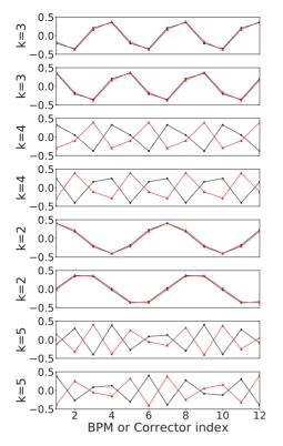
Figure 4: Columns of U (black) and V(red) matrices generated by SVD of simulated SIS18-ORM in y-plane.
