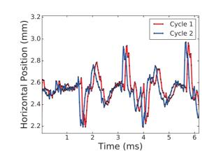
Figure 2: Measured horizontal position of two consecutive cycles at injection plateau.
