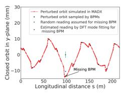
Figure 6: Closed orbit fitting in case of missing BPM.
