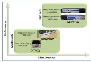
Figure 8: Hardware solutions according to performances requirements and cost.
