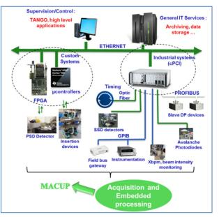
Figure 1: Acquisition and embedded process systems
