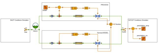
Figure 5: process model and nominal model simulation mock-up in EcosimProtm
