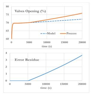
Figure 8: Environmental and sensor drift perturbation & error signature.
