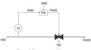
Figure 4: Pressure control loop.
