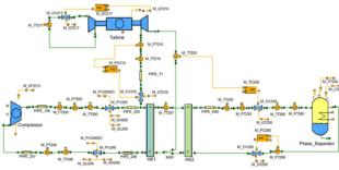
Figure 3: cryogenic plant overview in EcosimPro
