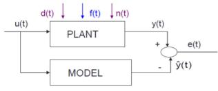
Figure 1: model based technique to perform fault detection analysing residues between measurements and a nominal model.
