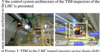
work Figure 3: TIM in the LHC tunnel passing sector doors (left) and the dimensions of one wagon (right).
