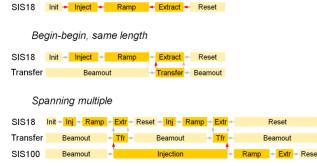
Figure 3: Relative scheduling of Beam Processes in LSA, example with booster mode and two injections into the SIS100.
