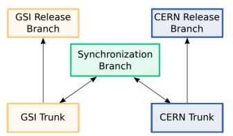
Figure 4: Repository setup including the new synchronization branch for feature exchange.
