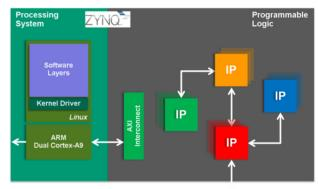
Figure 1: FPGA architecture.
