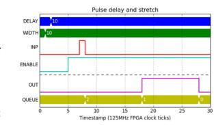
Figure 2: Generated signal diagram showing the output of a simulated pulse block. The output (OUT) is delayed by 10 counts and is stretched to have a width of 10.
