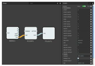
Figure 4: Screen shot of PandABlocks web GUI showing single input encoder block.
