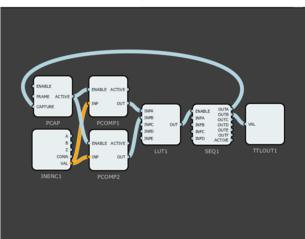
Figure 8: Block setup on web GUI for snake scan with time-based pulses.
