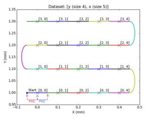
Figure 6: Snake scan with time based pulses.
