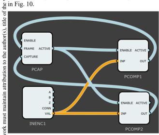
Figure 10: ADC Averaging block setup as seen on web GUI.
