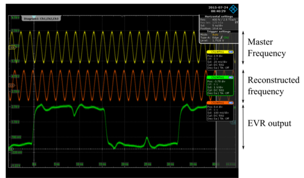
Figure 6: Laboratory proof of concept of the synchronism strategy using the timing system. A signal generator simulates de master frequency and an EVG-EVR pair generates the output triggers. Pulses of 31.25 MHz from the EVR output are used as a reference input for the second signal generator to create a 500 MHz sinusoid phase-locked to the master frequency.
