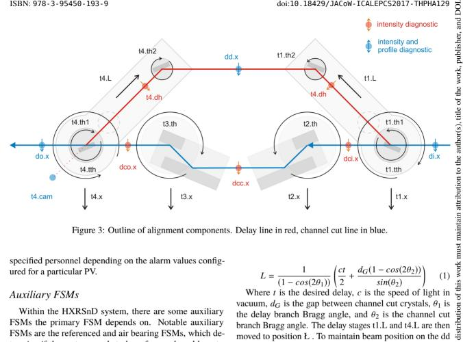
Figure 3: Outline of alignment components. Delay line in red, channel cut line in blue.
