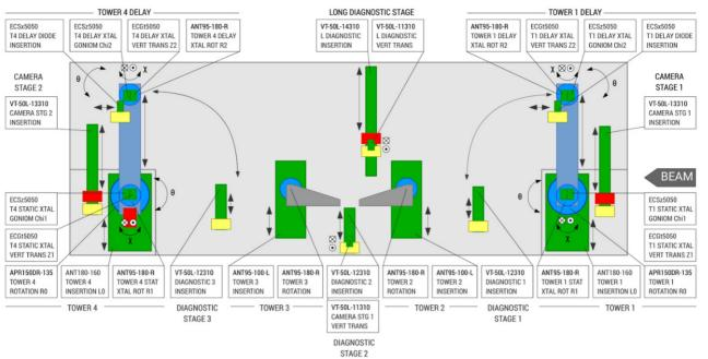
Figure 1: Detailed overview of the HXRSnD motion system for the towers and diagnostics.
