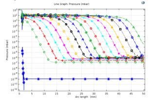
Figure 2: Distribution of pressure in a sample cell by time.
