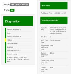
Figure 4: Fragment of the MARS UI showing the diagnostics information for a PLC.
