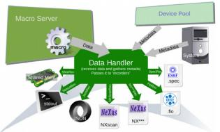
Figure 2: Sardana is driven by the data acquisition, managing data and metadata for data analysis and on-line information for control.
