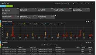
Figure 2: Kibana 3 user interface to the alarm data stored in Elasticsearch. The histogram shows the number of alarms over time, and the list at the bottom shows each individual alarm events. The dashboard is configured with some preset filters that can be activated to restrict the information shown in various ways. Custom searches on the various fields are also possible.
