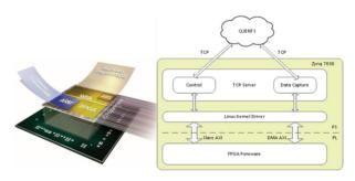
Figure 4: Zynq SoC firmware architecture.
