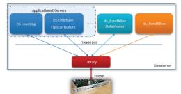
Figure 13: TANGO software architecture at SOLEIL.
