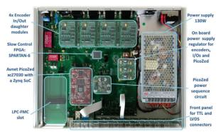
Figure 2: PandABox internal hardware top view.
