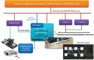
Figure 15: Continuous scanning synchronization with Pand-ABox.
