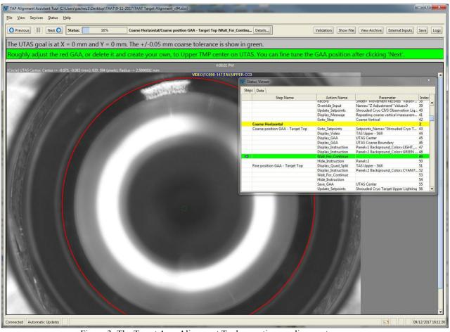
Figure 3: The Target Area Alignment Tool executing an alignment sequence.
