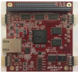
Figure 2: The Picture of the SoC IOC Board.
