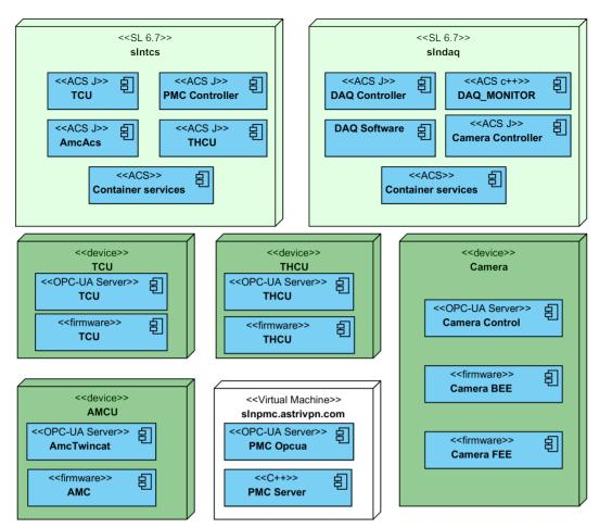
Figure 4: UML deployment diagram of the ASTRI telescope system.
