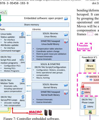
Figure 7: Controller embedded software.
