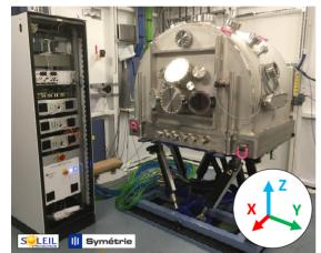
Figure 1: In vacuum diffractometer installed in the 20 SIRIUS beamline experimental hutch with its electronics the rack
