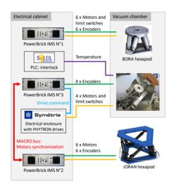
Figure 4: Hardware architecture.
