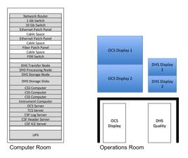
Figure 2: End to End hardware schematic.
