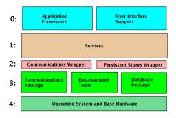
Figure 1: Layout of Common Services Framework.
