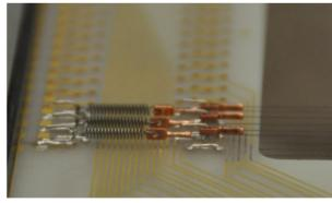
Figure 3: Spring loaded wires of Harp Head.
