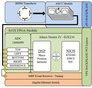
Figure 6: cPCi/VPX BPPM architecture.
