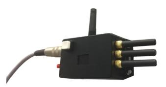
Figure 4: First generation operational node. External connector cable seen at left for RS-232 interface and external power. Internal 3xAAA battery holder for wireless operation is provided.
