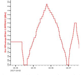
Figure 7: Measured data of power sweep for test received from wireless node and displayed in control system.
