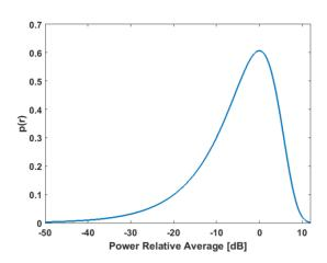
Figure 1: Probability Density Function (PDF) of expected signal variations of the measured signal power.
