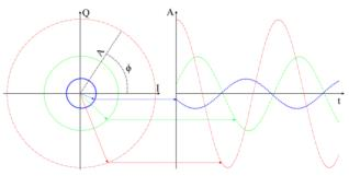
Figure 1: IQ modulation of a sine wave.
