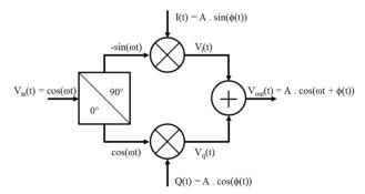
Figure 2: IQ modulator device schematic.
