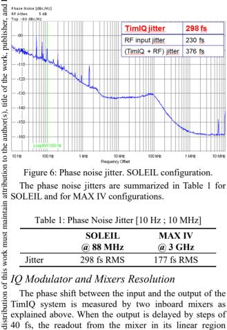
Figure 6: Phase noise jitter. SOLEIL configuration.
