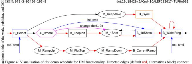
Figure 4: Visualization of *dot* demo schedule for DM functionality. Directed edges (default red, alternatives black) connect messages (ovals), commands (hexagon) to sequences terminated by time blocks (rectangles). Target (blue) and destination update edges (magenta) provide command context. Time blocks with command queues allow real-time changes (blue), sync time blocks auto-align to a given time grid (orange).
