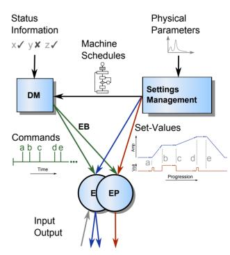
Figure 1: Schematic of FAIR CS. Left: Real-time Data Master (DM), Right: Settings Management Server. Endpoints (EP) receive both commands and set-values.
