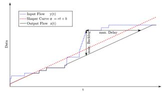
Figure 5: Network flow shaped by an arrival curve.
