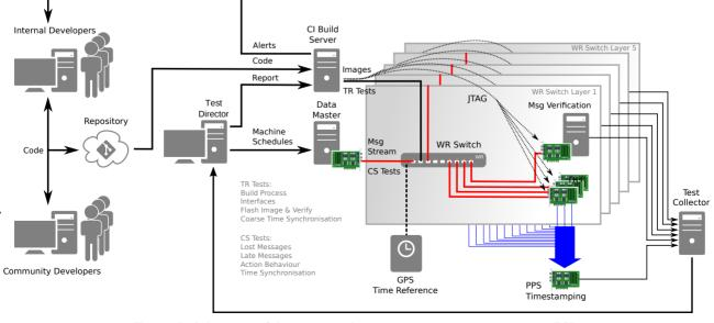
Figure 2: Schematic of the automated continuous integration system at GSI.
