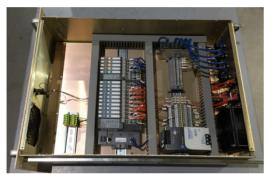
Figure 2: Vacuum interlock chassis module layout.
