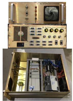
Figure 1: Intelligent Chassis Front/Rear Panel and Module Layout.
