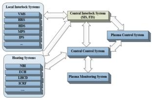
Figure 1: Interlock related system interface.
