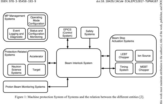
Figure 1: Machine protection System of Systems and the relation between the different entities [2].
