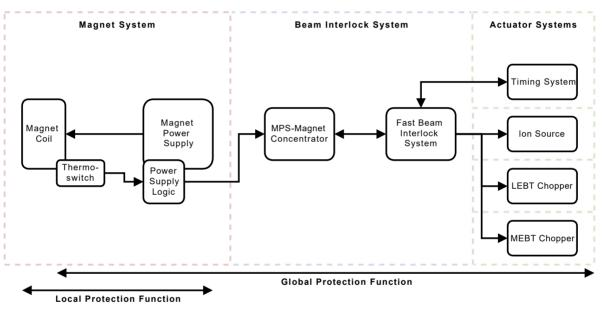
Figure 2: Example of a global and a local protection function at ESS.
