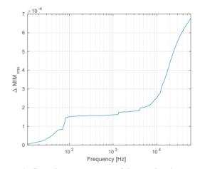
Figure 4: Cumulative spectrum of the amplitude error for a low beta cavity SEL driven.
