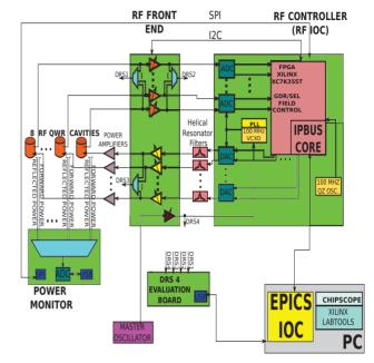
Figure 1: Block diagram of the LLRF system
