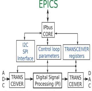
Figure 2: Block diagram of the firmware implemented.
