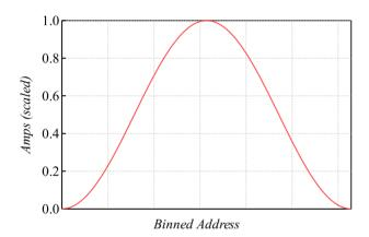
Figure 2: Offset sine wave trace used as the waveform in the power supply controllers. Using an offset prevents the supply from having to switch polarity which can potentially introduce switching noise.
