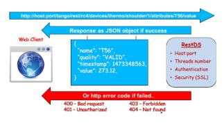
Figure 3: RestDS general operational diagram.
