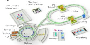
Figure 1: NICA accelerator complex general scheme [2].
