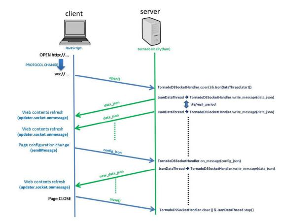
Figure 3: Communication flow between client and server for Tornado DS.
