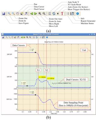
Figure 5: Plot page of vacuum interlock event. PosILK: position interlock, VacILK: vacuum interlock, MPSTrip: machine protection system sum trip, SRF3RC: SRF#3 ready chain signal, Pf: forward power, Pr: reflect power, GV: gap voltage.
