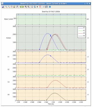
Figure 6: Kicker waveforms during spontaneous fired kickers K1, K3, and K4 while the K2 is misfired causing a beam trip.
