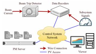
Figure 1: Schematic layout of the TPS PM system.
