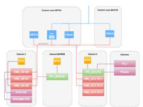
Figure 10: Network scheme of the Platform 704 MHz.
