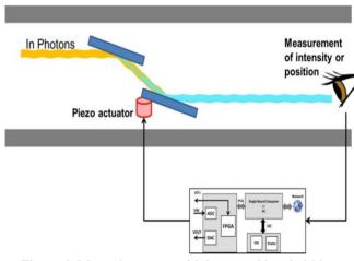
Figure 6: Monochromator with increased bandwidth.
