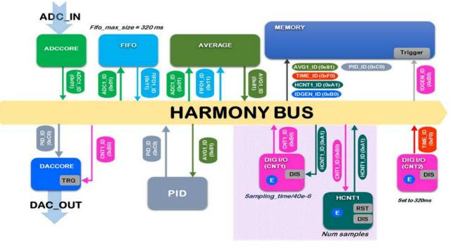
Figure 4: Harmony bus data flow for an acquisition on Em# project, using the Harmony Bus.
