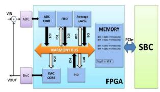
Figure 3: FPGA cores configuration with HB for a feedback system.
