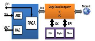
Figure 1: Electric block diagram of new ALBA development.
