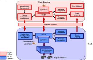
Figure 1: LMJ Software architecture.
